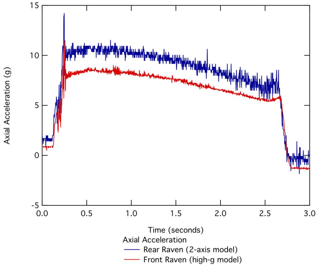
This plot is enlarged to show the thrust curves recorded; they are in agreement with the published thrust curve for the AT J540R motor, shown below.
